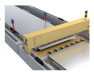
Web edge control of metal sheets with external synchronous evaluation
