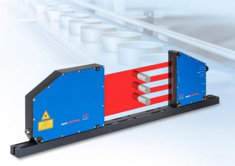
The optoCONTROL 2520-95 is a compact laser micrometer that features excellent linearity and high accuracy with a large measuring range of 95 mm. The optoCONTROL 2520-95 is flexible; the measuring object can be placed at any position within the light curtain and the distance from the light source to the receiver can be freely selected.
