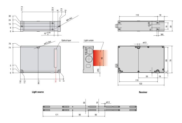
Light source and receiver with mounting rail
